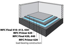
Levelling of industrial floors under synthetic coat
