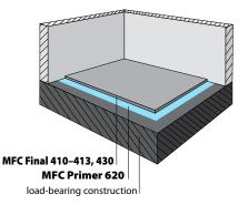
Surface treatment with final topping with underlayment screed during reconstruction of industrial fltoors
